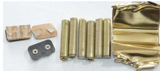
9V battery made up of 6 cells
